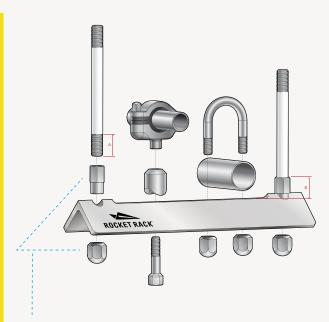
Specially-designed stainless mounting hardware supplied with tented angle, one set per mounting hole. (2 Beveled Cap Nuts and 2 Turned Rod Couplings) Please specify rod size – 3/8" or 1/2"
