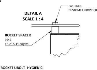
Minimal Thread Exposure 316S **DETAIL B** 1/2" - 4" Rigid Trade Size **SCALE 1:4** Includes: 2- RR BEVELED CAP NUT **ROCKET RACK BEVELED CAP NUT** 360° Nylon Thread Locker 316S
